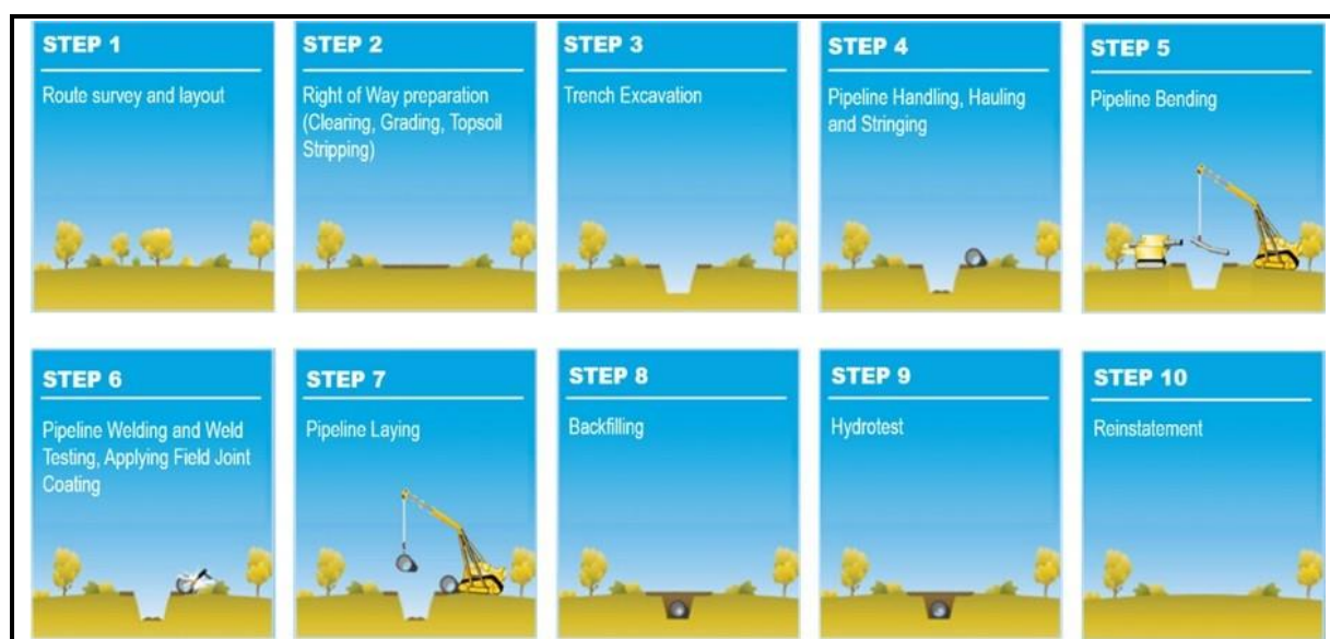
Figure 2-10 Typical Pipeline Construction Sequence
