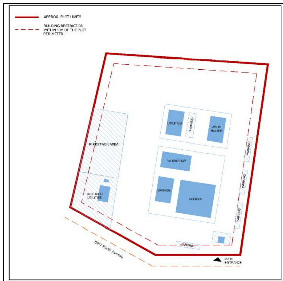
Figure 6-19 Indicative Preliminary Layout on Proposed Plot for Dispatching and O&M Centre
