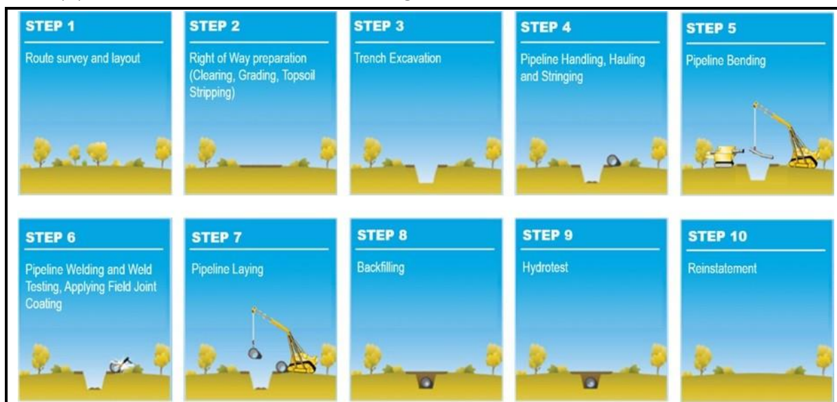
Figure 6-30 Typical Pipeline Construction Sequence
