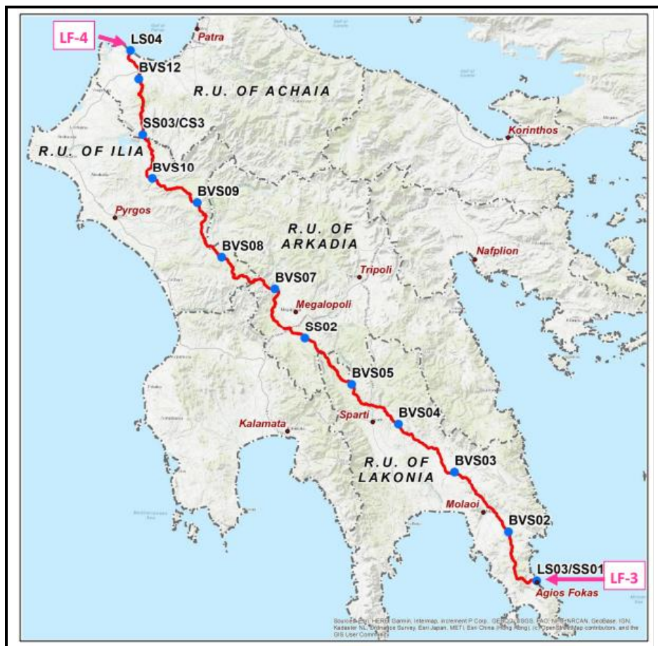
Figure 6-47 Overview of LSs, BVs and SSs locations along Onshore EastMed Pipeline – CCS1 Peloponnese Section
