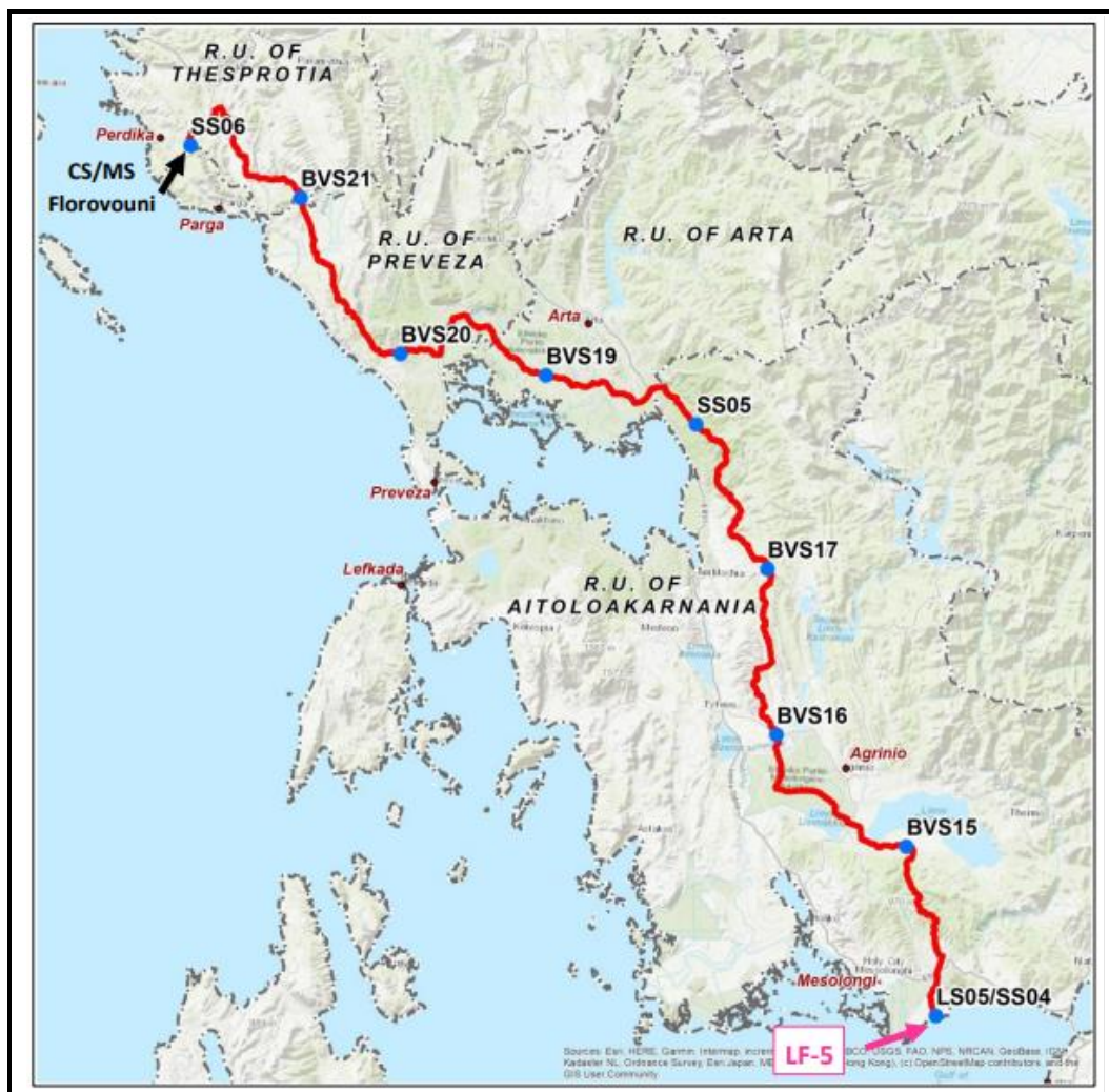
Figure 6-48 Overview of LSs, BVs and SSs locations along Onshore EastMed Pipeline – CCS2 West Greece Section
