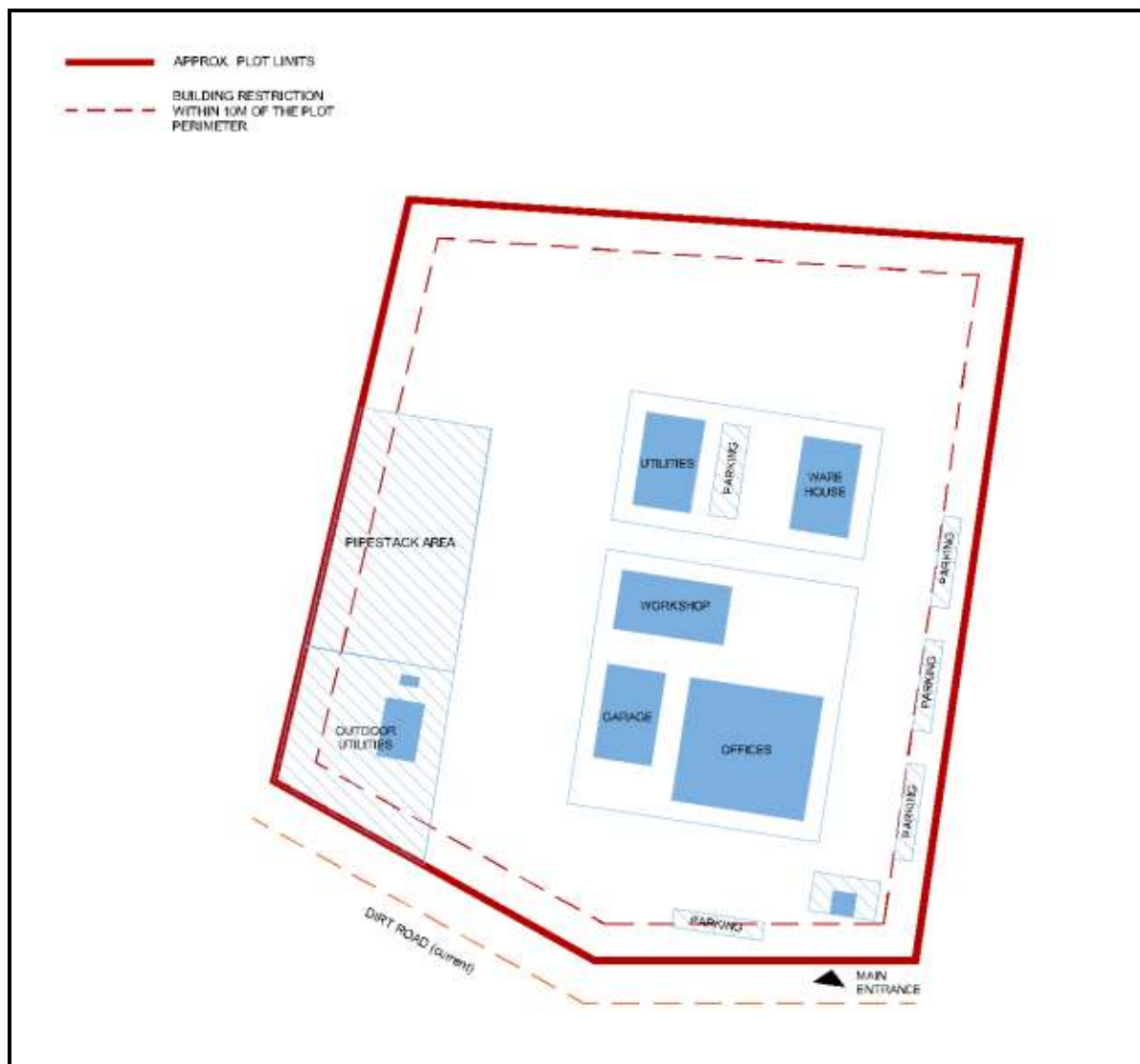
Figure 6-49 Schematic Layout of the Operation and Maintenance Base
