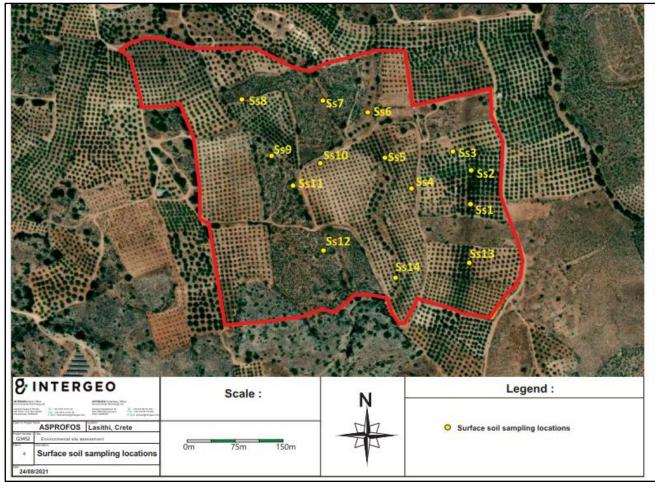
Figure 4 Surface soi sampling locations at the investigated plot in Lasithi, Crete
