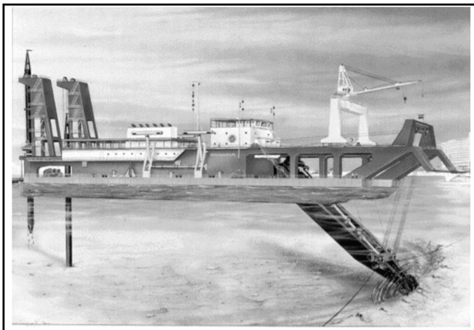
Figure D-8 Cutter Suction Dredger
