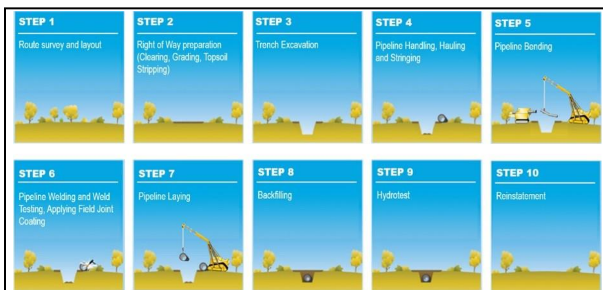
Figure 4-2 Typical Pipeline Construction Sequence
