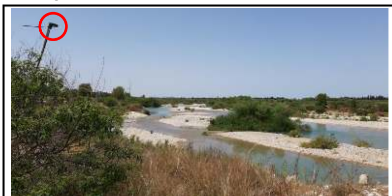
Figure 3-3 The microphone on the 3m pole that is connected with the SM4BAT-FS recorder at Evinos river.
