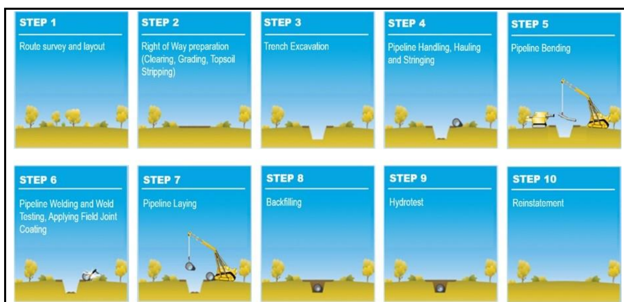
Figure 4-2 Typical Pipeline Construction Sequence
