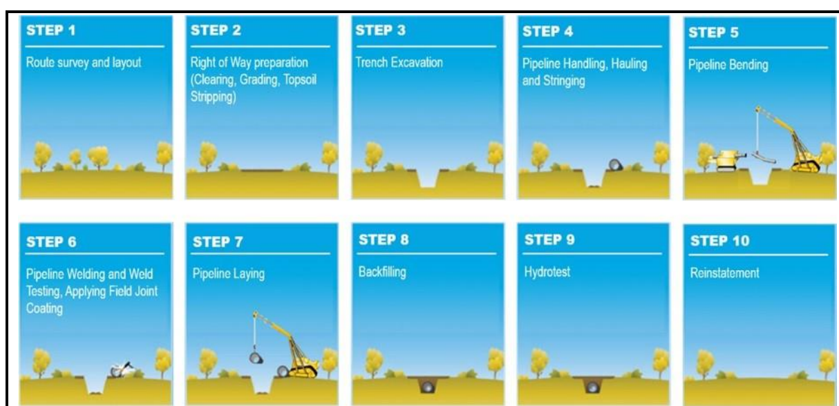
Figure 4-2 Typical Pipeline Construction Sequence
