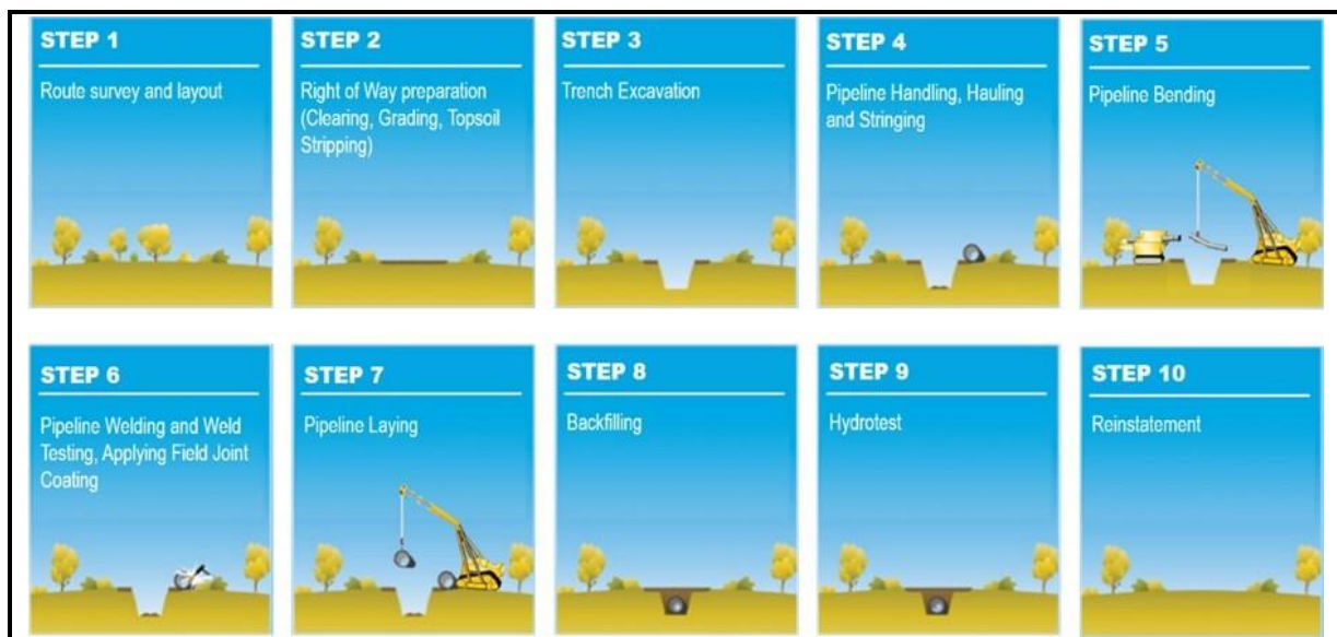
Figure 4-6 Typical Pipeline Construction Sequence
