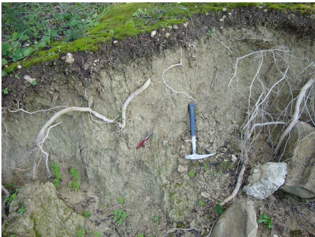
Photo 3: Field view of the Pliocene clay-marl sediments in the pipeline section A (site x/y: 180.492/4.358.881, Greek Grid)
